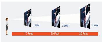
Pixel pitch is the distance from the center of a pixel to the center of any adjacent one. The smaller the pixel pitch, the higher the density and the clearer the image. Greater pixel density carries a higher price tag, so the best way to choose the right option is to consider the optimal viewing distance for the type of content - whether its text, images or video; and its application - whether for company presentations or for digital signage.
